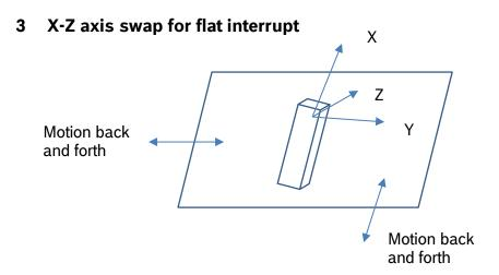
If the device is sitting on a surface with Z and Y axes flat, while X axis is pointing to sky or down, you can set BMA253 register 0x2D bit-7 to "1". Then for flat interrupt engine, X axis will become Z' and Z axis becomes X'. Therefore, the flat interrupt zone still works the same way.
