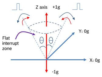
When Z axis is moving within the zone or out of the zone, there will be no more flat interrupts generated. Due to vibration or swing motions, Z axis acceleration data may change a lot which means that Z axis can exit the zone or enter the zone easily. But if the duration of the flat hold time is set to 0ms, then there may be some false interrupts. If it is set to 512ms, then flat interrupt is very robust.
