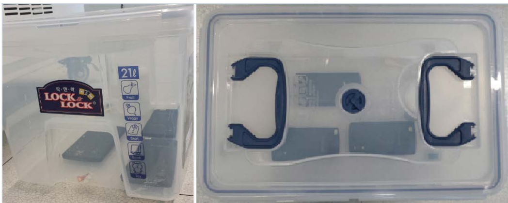
Figure 1: One example of an air tight box used for reference salt test: Lock & Lock
