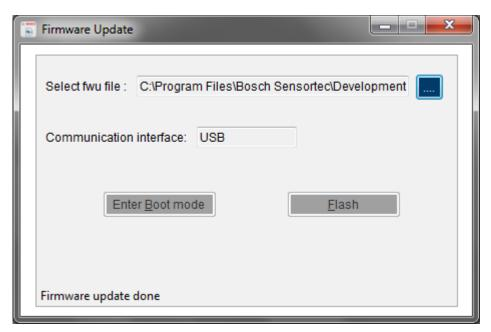
Step 9: Switch off the APP2.0 board and then switch it on. Restart the DD2.0\_UI3.20 GUI SW. It should work properly as shown below.
