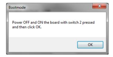
Step 6: The On/Off switch and switch 2 pushbutton are located on the APP2.0 board as shown below. Power off and then power on the APP2.0 board with switch 2 pressed. Then click OK button and then release switch 2.
